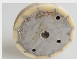
Test specimen: a metal holder inside the wheel. The individual segments of the "tyre" consist of the VarseoSmile Crown<sup>plus</sup> with a sealed surface.
