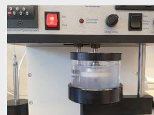
Test device for abrasion: there is a closed glass vessel in the lower half containing the test specimen immersed in a fluid with an abrasion agent.
